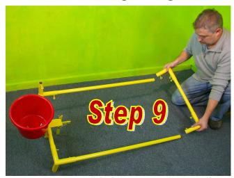
Place the remaining two corner fittings onto either end of the 24" pipe. Be sure to slide them completely on, but do not tighten. Attached these corner fittings to the opposite ends of the 41.5" pipes. (Leaving the corner fittings loose will help to guide them onto the pipes.) Tighten all fittings.
