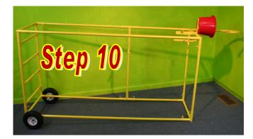
Tip the unit onto its side. Block the tires and find items to elevate the unit about a foot or so. Place the top on the unit, and tighten.
