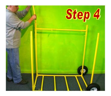
Insert a 41.5" pipe onto each tapered pipe.
