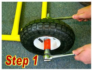
Attach tires to the base unit, with the 5/8" bolt and lock nut. (The nut goes on the inside side of the tire.)
