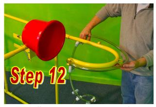
Attach filler tube. Use the clips to route the filler tube along the frame.
