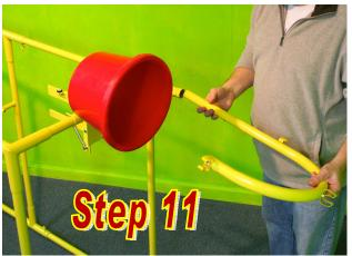
Insert filler tube hook and tighten.
