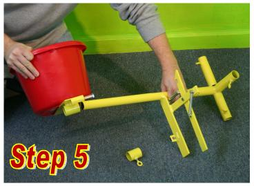
Slide the bucket assembly onto the trigger unit. Make sure that it is positioned so that the roller engages with the trigger hook.
